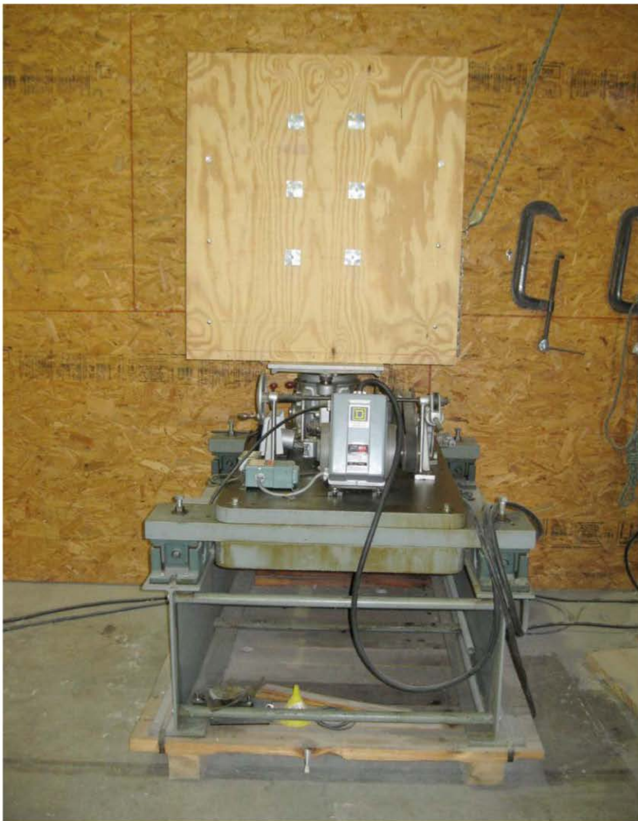
FIG. S7.2 Vibration Machine
